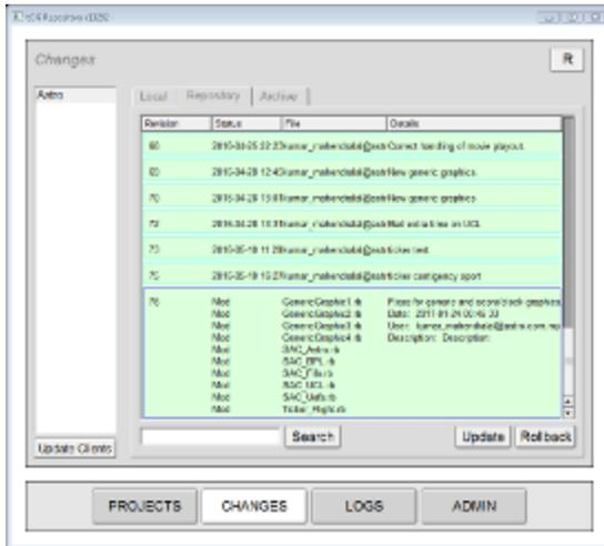
tOG Repository is used to maintain a “versioned database” of graphic templates (and associated assets) where each change is logged and to distribute the latest version of these graphics to an editable list of client machines - in the newsroom case this would be the central data server and all the rendering machines.
