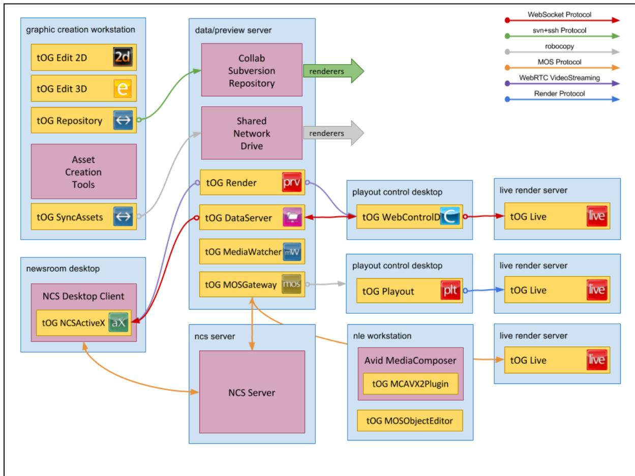
Data and control flow in the diagram above moves from left to right. On the left designers, producers and journalists create graphic templates and running orders (which reference the graphic templates). These assets are stored in the servers in the centre which distribute them to the section of playout and render machines on the right.
