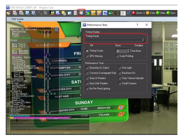
Sliding the "Timing Detail" to the far right brings up a column of timing data. The bottom value (Total) should be a constant 20ms (for 50Hz video) or 16.7ms (for 59.94Hz video). This is the total time taken to render a single frame (or field with interlaced video). If it exceeds 20 (or 16.7) then the system is not rendering in real time and the output will judder.
